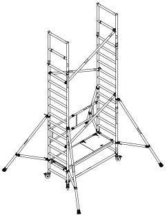
**9** Reposition the trapdoor deck as shown. From the protected trapdoor position, fit horizontal braces as shown.
