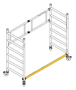
Fit 2 rung guardrail frames as shown. Fit diagonal brace in position shown.
