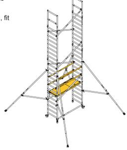
Fit the trapdoor deck as shown. From the protected trapdoor position, fit horizontal braces as shown.
