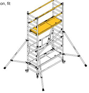
7 Fit 2 rung guardrail frames as shown. Fit diagonal braces in position shown.
