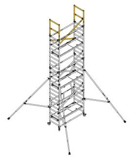
Reposition trapdoor decks and horizontal braces.
