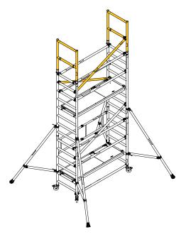
Reposition trapdoor decks and horizontal braces.
